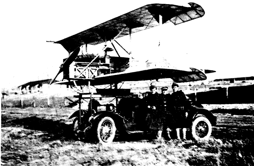
AN AUTOMOBILE IS SUBSTITUTED FOR A WIND TUNNEL IN A TEST OF A FLYING BOMB
